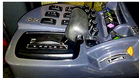
Gearbox control on fingertip platform
